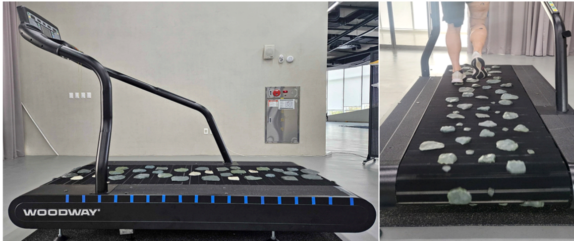
Figure 1. Modified treadmill surface for uneven terrain simulation
